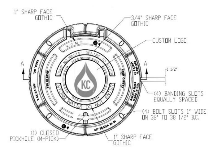
Figure 1: Standard Stormwater Markings
