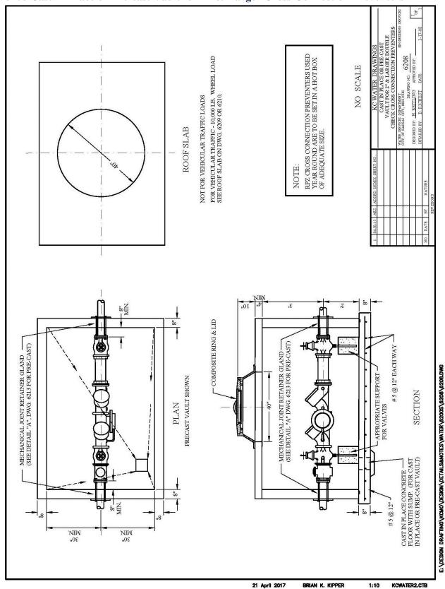
6209 Cast-in-Place or Pre-cast Meter Pit & Setting with Bypass for Single 3" thru 10" Meters
