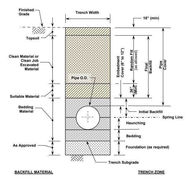
Figure 2. Trench Detail, Class A Bedding, Unpaved Areas
