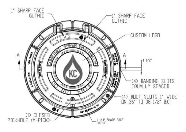
Figure 2: Optional Sanitary Sewer Manhole Markings
