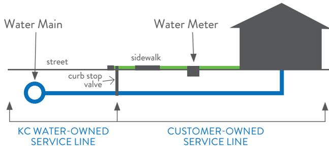
To continue assuring the safety of the Kansas City’s drinking water supply, KC Water is undertaking this initiative to identify materials used in service lines across the city. Service lines are the pipes that connect from water main pipes to buildings and houses (see graphic).
