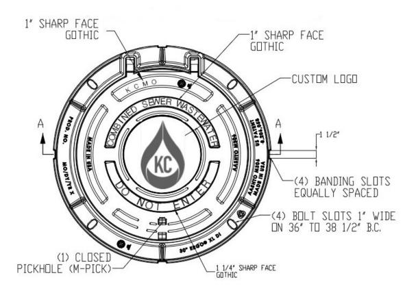
Figure 2: Optional Sanitary Sewer Manhole Markings
