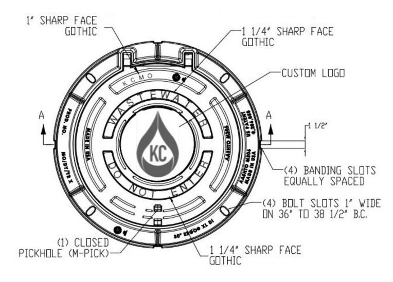
Figure 1: Standard Sanitary Sewer Manhole Markings For Ductile Iron Castings
