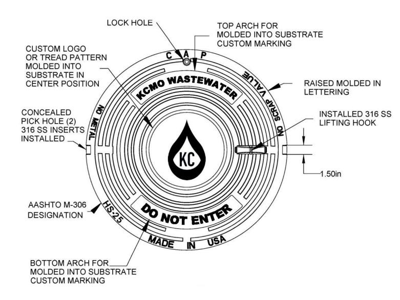
Figure 3: Standard Sanitary Sewer Manhole Markings For Composite Castings
